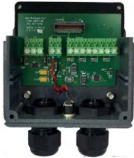
The 4x Analog Output includes four, 0-5 Vdc analog output ports. Analog outputs are fully scalable over the 0-5 Vdc output range for minimum and maximum voltage output. Module also includes two dual purpose switch I/O's for either input switch sensing or output switch control.
