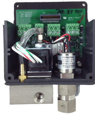
P/N 9203-2031052 AeroMate front cover assembly and 1x1 valve module shown disassembled. Front cover assembly, shown with wireless kit, is easily removed for routine valve maintenance.
